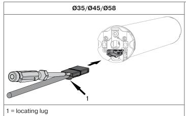
Insert the **dead** connecting cable into the drive head until the locating lug clicks into place in the drive. If necessary, use a suitable flathead screwdriver to assist with insertion. Set the screwdriver into one of the two plug grooves provided for this purpose.
