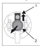
When pushed in, the mounting pin (2) locks automatically. To undo the mounting pin (2), push the tab washer (1) upwards and pull out the mounting pin (2).
