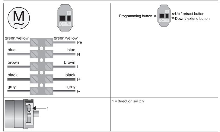
Connect the wires of the tubular drive to those of the same colour in the programming unit (Item No. 4935 200 034 0) and switch on the power supply.
