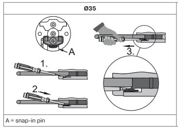
Insert a suitable flathead screwdriver between the locating lug and the snap-in pin, so that the snap-in pin releases the locating lug from the plug.
