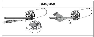
Insert a suitable flathead screwdriver right into the recess of the locating latch, so that the latch releases the locating lug from the plug.
