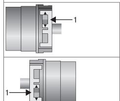
Switch the direction switch (1) to the opposite position.
